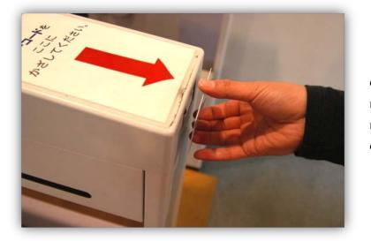
\* You may find ID reader a little bit cranky! Do not hold card too close to reader. Instead, hold card about 5 mm from reader and slightly move it to & fro and up & down.
